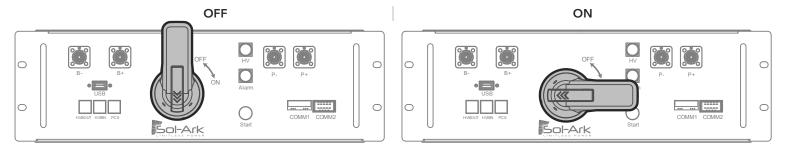
Figure 14 Operation of the BMU DC Disconnect
