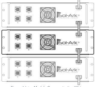
Figure 6 Inter-Module Communication Wiring
