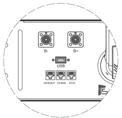
Figure 7 Battery Module Communication Ports
