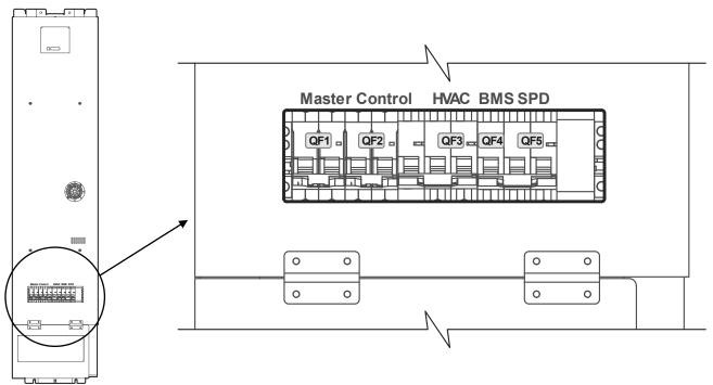
Figure 12 Location of the Control Systems Breakers
