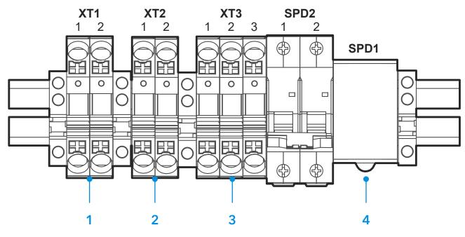
Figure 8 Auxiliary Wiring Terminal Block
