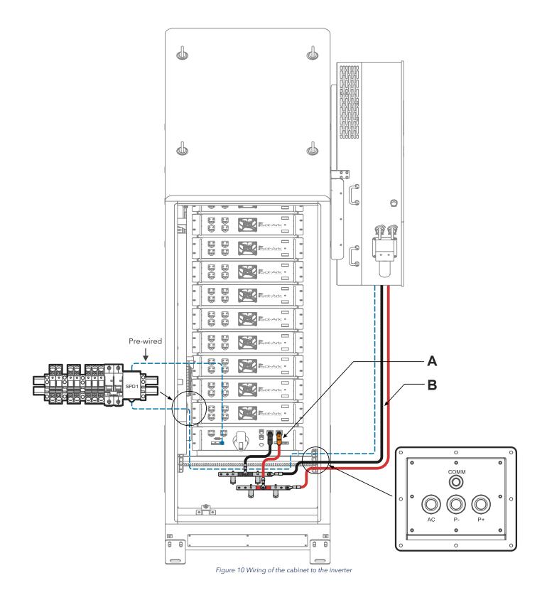
🌔 Please note that 2x 9.8ft (300cm) cables are included in the shipment for the *"B"* connection shown above (battery busbar to Sol-Ark inverter).
