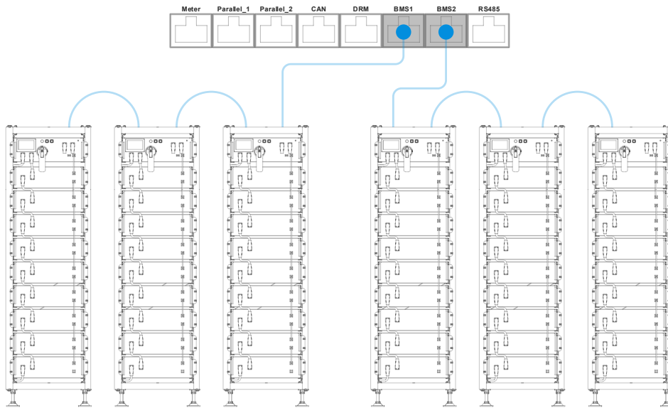
Figure 7: Multi-Battery Bank Communications
