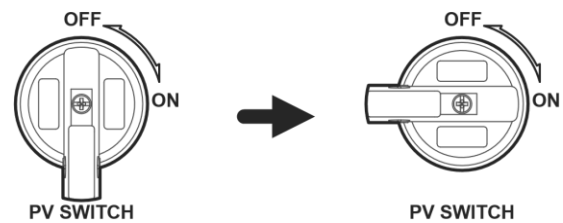
Figure 17: PV Disconnect Operation
