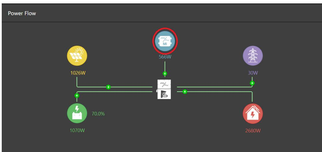
If AC coupling is not set up through the **GEN** terminal, then an accurate reading of your AC coupled solution is not available, because loads in conjunction with your AC coupled solution can pull power that the solution supplies.
