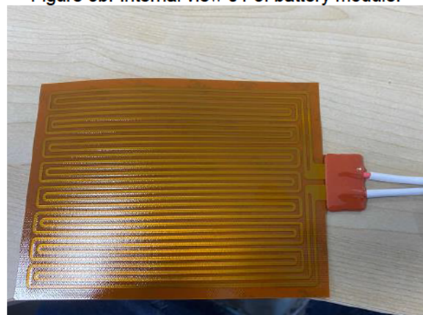
Figure 5d. View of heater.
