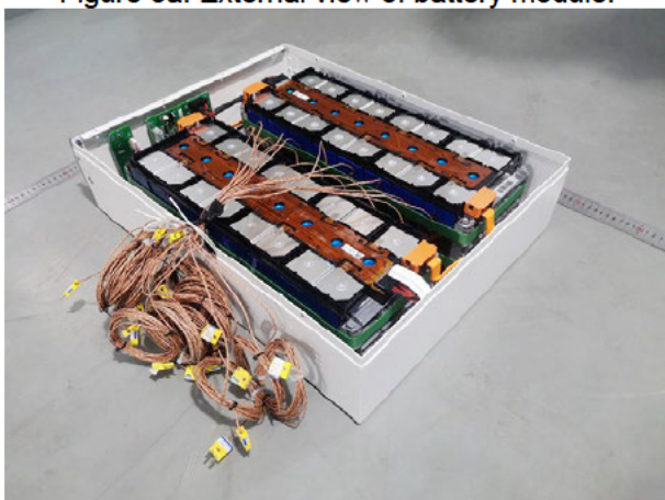
Figure 5c. Internal view 02 of battery module.
