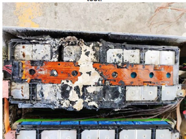
Figure 21d. Photo 02 of thermal runaway location.
