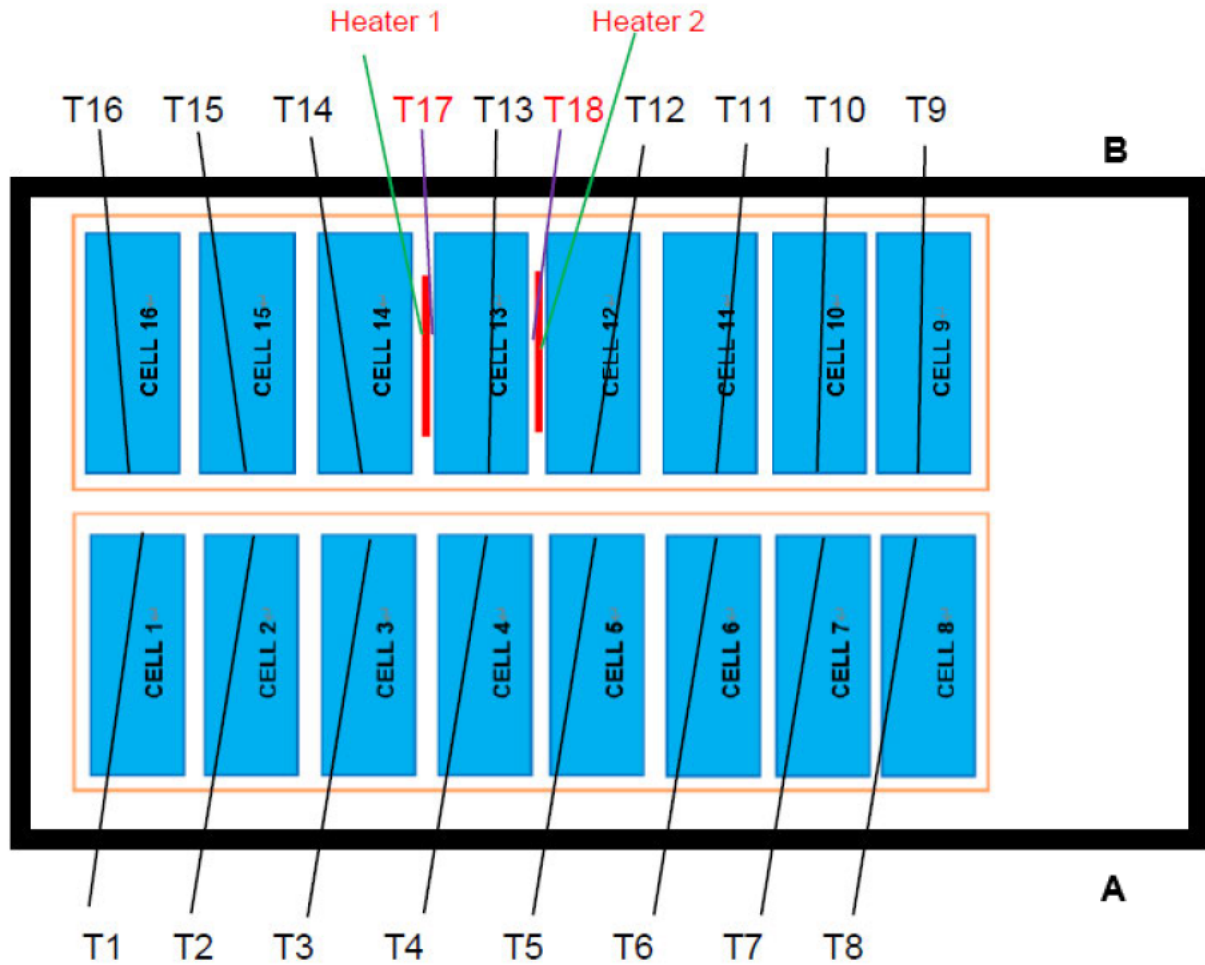
Figure 6. Schematic diagram of external heater and thermocouple locations in the initiating module (View from top).
