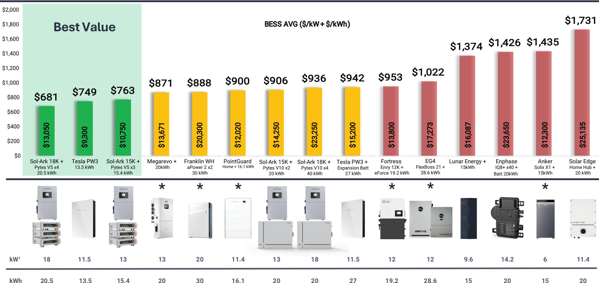
BESS AVG (\$/kW + \$/kWh) accounts for the system power (AKA engine) and energy capacity (AKA gas tank)
